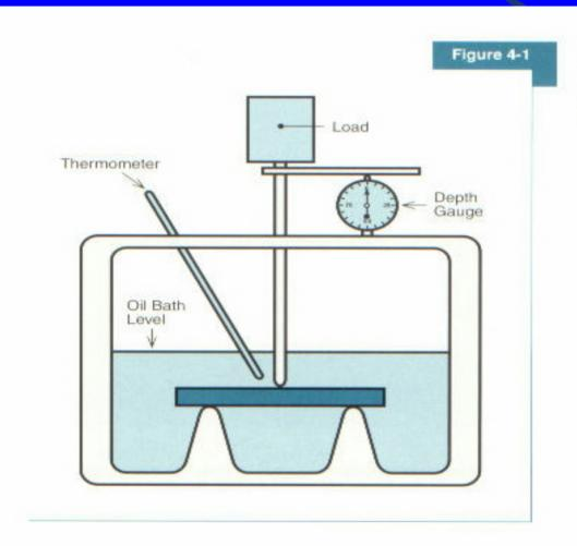
Test apparatus for deflection temperature under load (DTUL).
