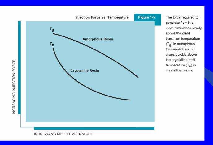
Because of these easier flow characteristics, crystalline resins have an advantage in filling thin-walled sections, as in electrical connectors.
